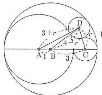
$$\overline{AD} = 3 + r_2 \text{ (외접)}, \quad \overline{CD} = 1 + r_2 \text{ (외접)}, \quad \overline{BD} = 4 - r_2 \text{ (내접)이고}$$
